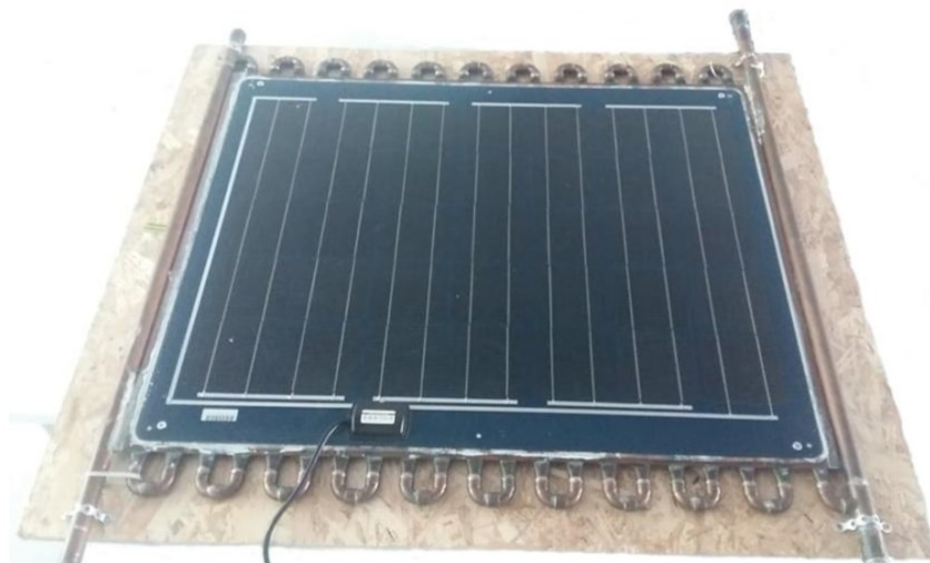
Figure 1. Photovoltaic Solar Collector
